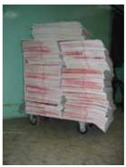
100 semi-products are bound together with a plastic threat. First 2-3 sheets on each side are bent and cannot be further processed (loss of 6 % of semi-products!). Paper piles are tipped over in the storage area. Papers are stored and transported on inappropriate devices or bend during transport.
