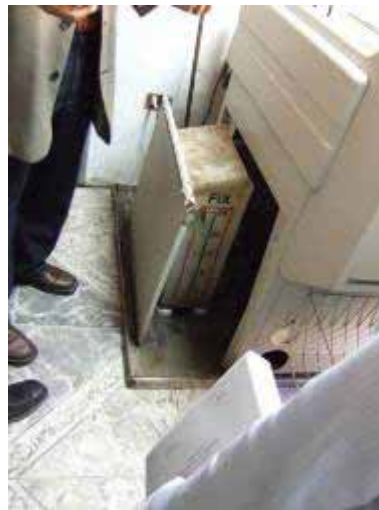
containers for fresh and used fixer (or developer) need to be frequently refilled.
