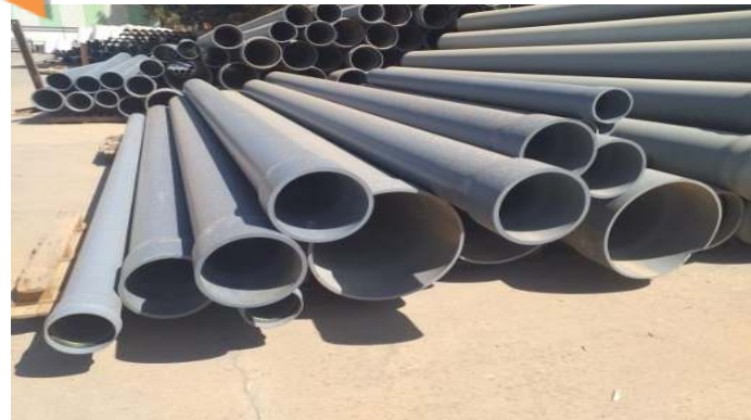
Tubes PVC conformes
